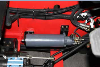
There's an energy accumulator applied in the braking system, which means when the engine is shut down,it can also provides more than 4 times emergency brake.
