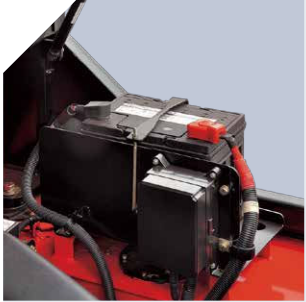
All the controllers,relays,and safety fuses are allocated in the controller box, free to water and dust. The main electronic components are waterproof, which is capable operator in severe enviroment. And the famous brand air-filter is also applied in the truck.
