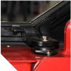
There're four levels shock absorption applied to reduced the vibration from the road to the driver. The damping pad is applied reduce the vibration, Like between the steering axle and the chassis, The engine, torque convertor and the chassis, the overhead guard and the chassis. And the suspension seat is another vibration reduction.
