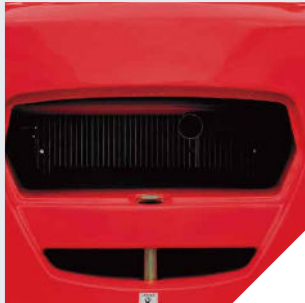
The patent plated-fin type aluminum radiator is applied,the heat exchanging is approved,and improves the capability for operation in severe environments.
