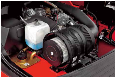
The new stamped air cleaner featuring tangential intake, double seal with safety filter is durable, corrosion-free and vibration-resistant, provides better filter efficiency and lower intake resistance than the previous.
