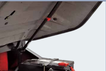
The locking device of the engine hood damper and parking brake help add to safety.
